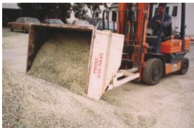
Crushed recycled glass at the Recovered Materials Foundation. This is being used in a variety of products like Blast Glass, Glass Crete, Filter Crystal and Architectural Coatings.
